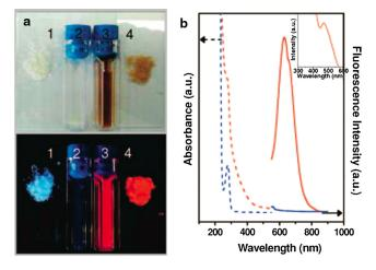
**Fig. 5** Comparison between BSA (blue) and red-emitting BSA-Au NC (red), both in solution and in lyophilized form. The absorption spectra are the dashed lines and fluorescence spectra are the solid lines. Inset image is the excitation spectrum of BSA-Au NC. See Ref. 48).
