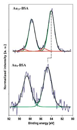
**Fig. 3** XPS spectra of the Au 4f band for BSA-Au<sub>25</sub> and BSA-Au<sub>8</sub>. A shift in higher binding energy is seen for smaller clusters. From peak fitting of each band, mostly  $Au^0$  is only seen for  $Au_8$  where  $Au_{25}$  has some  $Au^+$  contribution, likely from the NC surface. (See Ref. 55).
