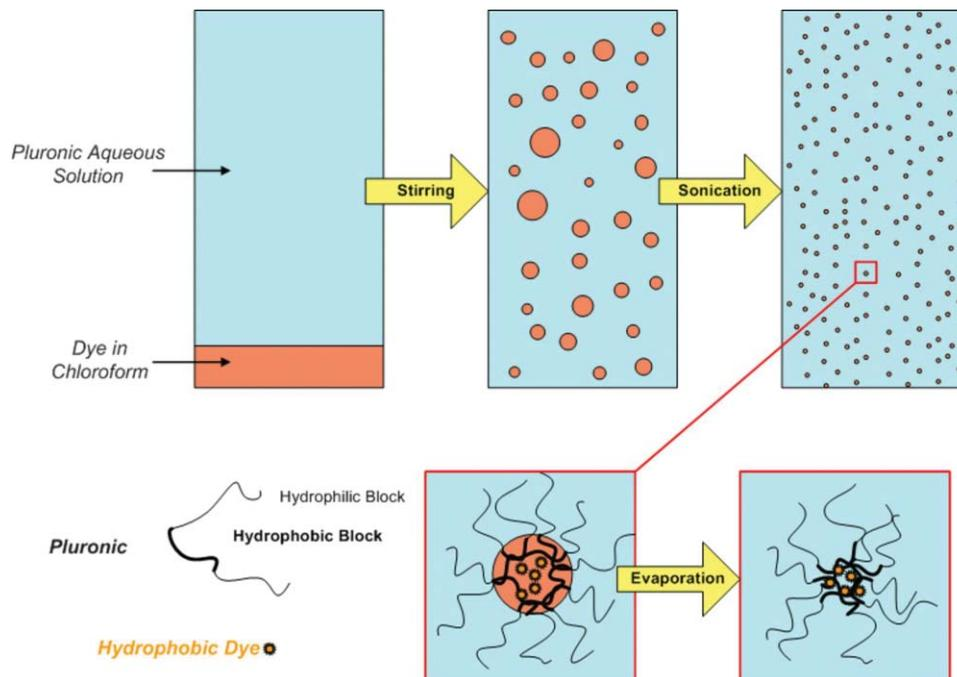
Fig. 2 Schematic representation of the Pluronic micelles synthesis (see text for details).
