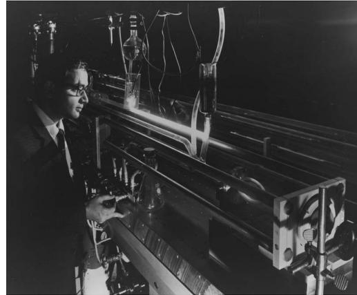
**Fig. 10** Kumar Patel with a flowing-gas CO<sub>2</sub> laser in 1967. (Courtesy of Bell Labs)
