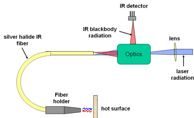
**Fig. 1** The single-fiber laser bonding system. A simple optical setup focuses the  $CO_2$  laser beam onto the proximal end of the fiber, and the blackbody infrared (IR) radiation emitted from the heated spot is collected by the same fiber and transmitted back towards the IR detector.
