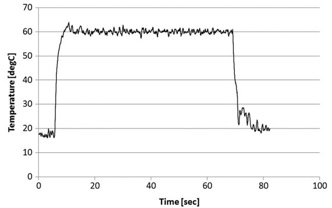
**Fig. 3** Temperature monitoring and control of a heated spot on a bovine cornea. The set value was reached within  $\sim 5$  s. There is hardly any overshoot.
