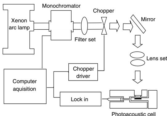
Fig. 1 Experimental setup of the used PAS.
