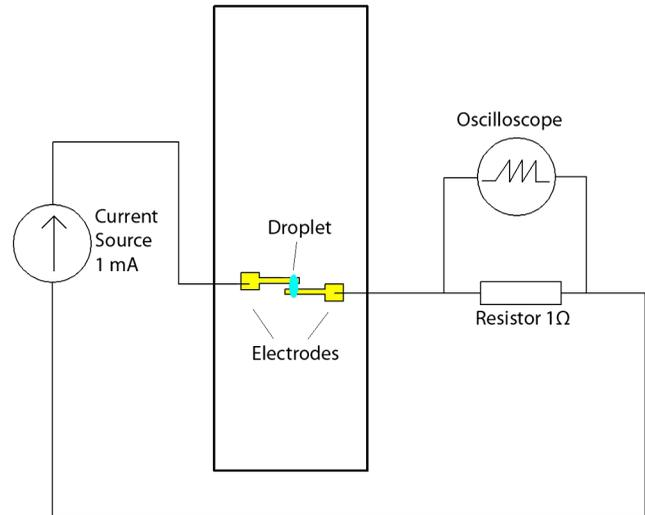
**Fig. 13** Schematic diagram of the droplet-counting circuit for the demonstrated microfluidics system.
