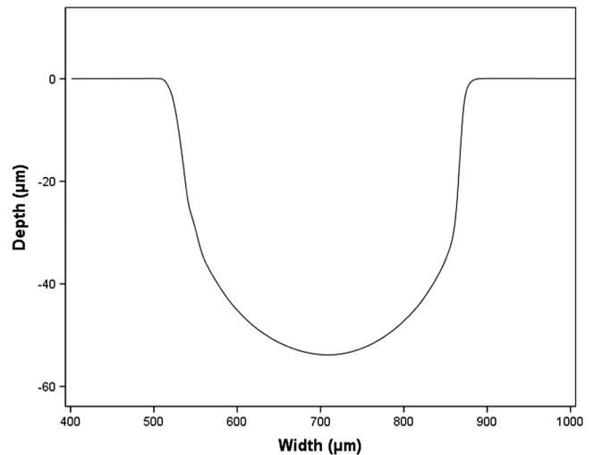
Fig. 10 Profile measurement of the microfluidic channel on a 1-mm PMMA sheet after the deep-UV exposure and development.
