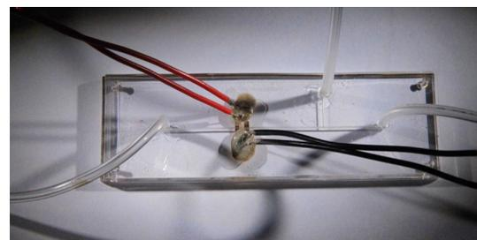
**Fig. 3** The microfluidic system with T-shaped microfluidic channels and electrodes after the fabrication process.
