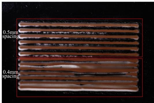
**Fig. 5** The warping of plastic paper during the laser cutting on plastic paper. Minimum spacing of the cut line is 0.5 mm to avoid warping.
