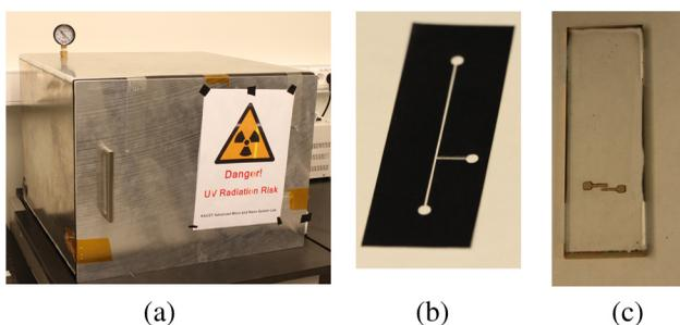
**Fig. 2** (a) Custom-made 254-nm deep-UV exposure box. (b) Laser-patterned wax-covered plastic paper used as a mask for the patterning of the microfluidic channel. (c) PMMA sheet after Au sputtering using the wax-covered plastic paper mask.
