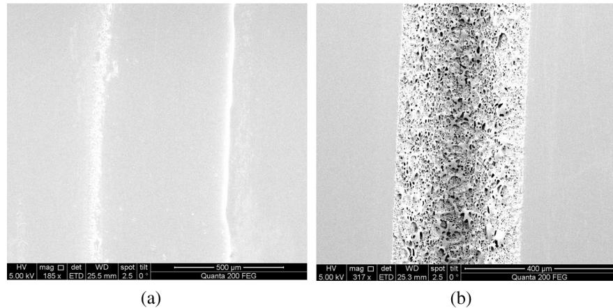
Fig. 8 SEM images of (a) the deep-UV fabricated channels on a 1-mm thick PMMA sheet and (b) laser-ablated microchannels on PMMA sheet.
