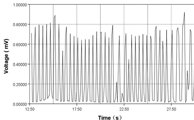
**Fig. 14** Signal measurement of the demonstrated microfluidics system, each peak represents a droplet passing through the electrodes.
