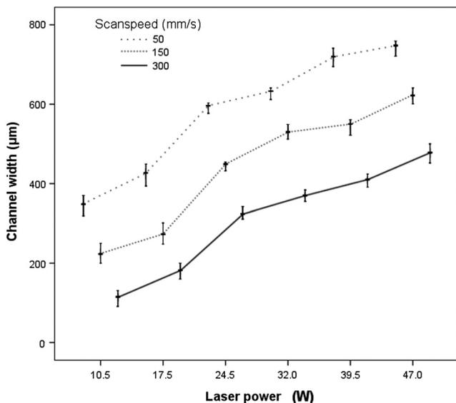
**Fig. 12** Channel width comparison of the laser-ablated microchannels with various laser scan speeds and powers.
