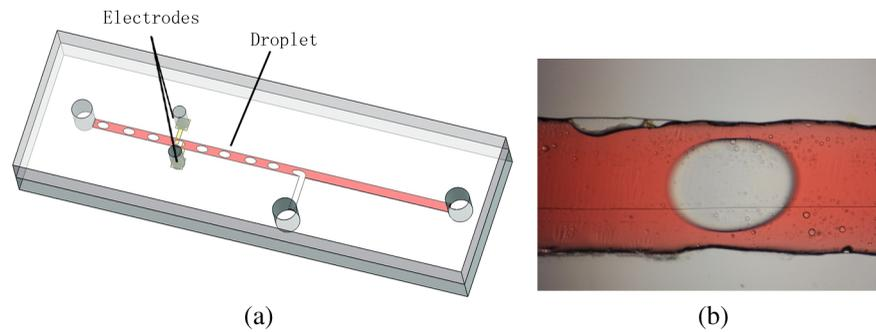
**Fig. 4** (a) Schematic diagram of the microfluidic system for droplet generation and detection. (b) Image of an oil droplet in a red-dyed water carrier generated in the PMMA microchannel.
