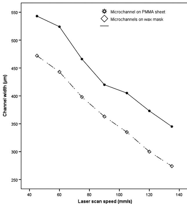
Fig. 9 Undercut during the deep-UV patterning of PMMA sheet.
