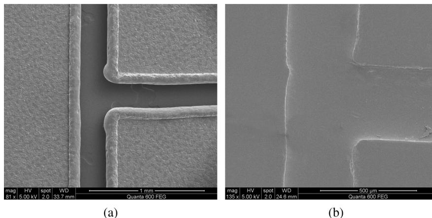
**Fig. 6** (a) The laser-cut patterns on wax-covered plastic paper. (b) Corresponding areas (junction of microfluidics channels) on PMMA sheet after development.
