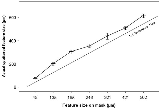
**Fig. 11** Comparison of the mask feature size and actual patterned (Au sputtering) feature size with the 1:1 reference line.
