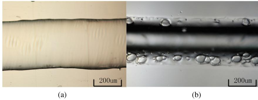
Fig. 7 Optical images of (a) the deep-UV fabricated channels on a 1-mm thick PMMA sheet and (b) laser-ablated microchannels on PMMA sheet.
