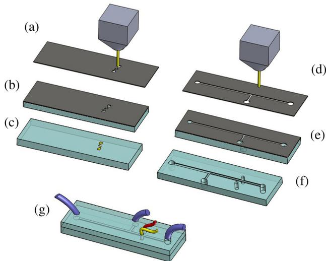
**Fig. 1** Fabrication process of a polymethylmethacrylate (PMMA)-based microfluidic system using laser-patterned wax masks. (a) Laser cutting of the wax-covered plastic paper, which works as a mask for sputtering. (b) Sputtering Au (50 nm). (c) Removal of the wax mask. (d) Laser cutting of the wax-coated plastic paper, which works as the mask for 254-nm deep-UV patterning. (e) Deep-UV exposure of PMMA. (f) The PMMA sheet after UV exposure and development. (g) Bonding, piping, and wiring.
