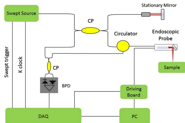
**Fig. 2** MEMS-based endoscopic SS-OCT system. CP:  $2 \times 2$  fiber coupler; BPD: balanced photo detector; Control Board: output scan driving signal to probe and sync signal to DAQ board for data acquiring.
