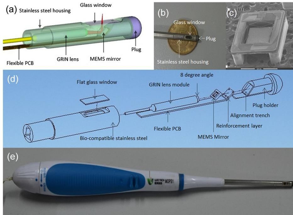
**Fig. 1** (a) Three-dimensional (3-D) model of the MEMS-based endoscopic probe; (b) a photo of an assembled probe; (c) dual S-shape bimorph MEMS mirror; (d) exploded view of the probe assembly; and (e) the complete handheld OCT probe (210 mm long).
