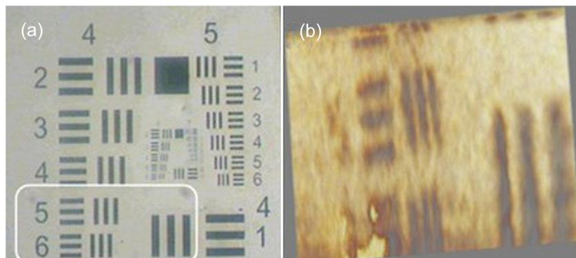
**Fig. 4** Resolution test. Group 4 element 6 (a) can be identified in OCT image (b).
