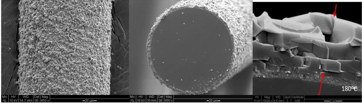
Figure 3: SEM images of the multilayer coated long period fiber grating silicalite and SCZY films for hydrogen detection at temperatures near 500°C.
