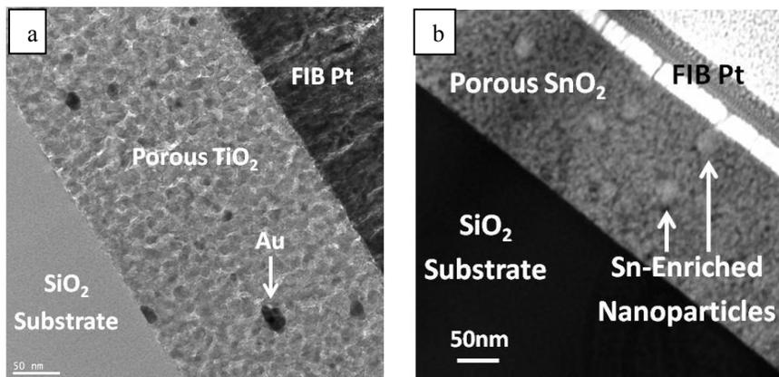
Figure 6: a) Au Incorporated TiO<sub>2</sub> Film Calcined at 500°C, and b) SnO<sub>2</sub> Thin Film After H<sub>2</sub> Exposure to Show Formation of Sn-Enriched Nanoparticles
