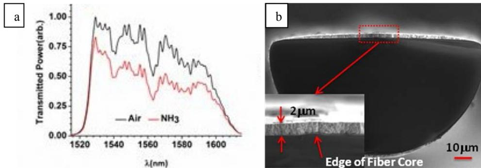
Figure 7: a) Wavelength spectra of Ammonia Detection in air using a SnO<sub>2</sub> doped nanocomposite, and b) SEM of coated optical fiber with metal oxide composite.
