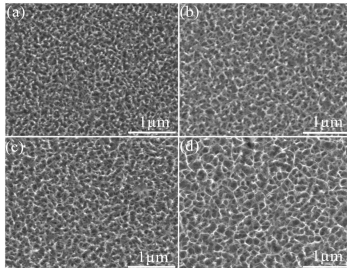
Figure 4: SEM images of the  $\text{TiO}_2$  nanoporous films synthesized at different temperatures: (a)  $80^\circ\text{C}$ ; (b)  $120^\circ\text{C}$ , (c)  $160^\circ\text{C}$ , and (d)  $200^\circ\text{C}$ , respectively.
