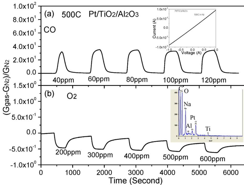
Figure 5: The sensitivity of Pt coated TiO<sub>2</sub> nanoporous film measured at 500°C in (a) CO and (b) O<sub>2</sub> with different contents. The inset of (a) shows the I-V curve at 500°C in N<sub>2</sub> atmosphere. The inset of (b) shows the Energy Dispersive Spectroscopy (EDS) spectrum of Pt coated TiO<sub>2</sub> nanoporous film.
