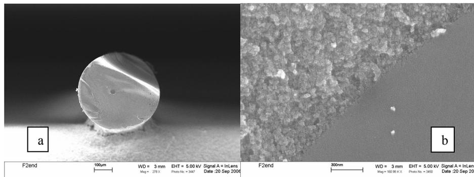
Figure 8: SEM image of porous nanostructured fiber with a) face of fiber showing porous cladding and solid core, and b) showing interface of core and porous cladding.
