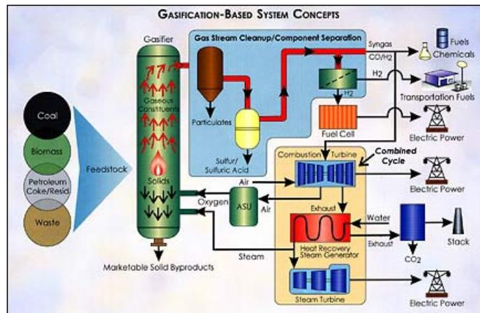
Figure 1: Advanced Concepts in Integrated Gasification Combine Cycle Power Plants
