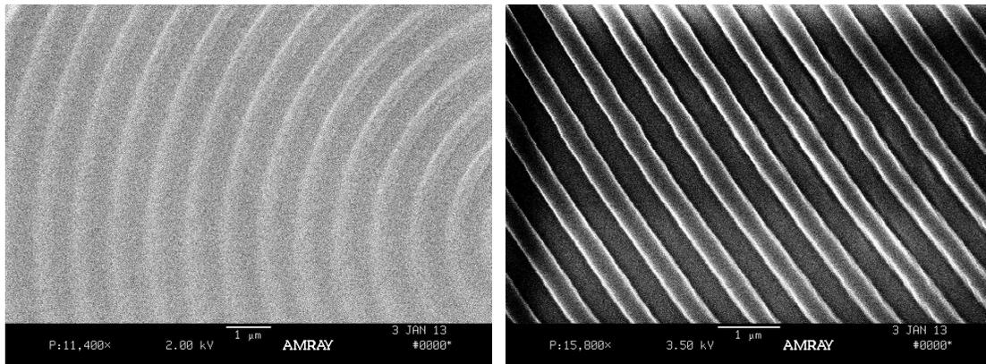
Figure 2: SEM images of a “bull’s-eye” energy harvesting plasmonic device under development by the University of New York at Albany and University of Minnesota.
