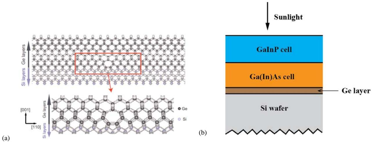
Figure 4. (a) “Lattice matching in a monolayer” – lowest energy configuration for Ge on Si, once more than 12 monolayers deposited (after [3]); (b) “Out-of-sequence” tandem. Photons are shared between the Si and Ge, with rear light-trapping features increasing Ge absorption of photons below the Si bandgap.
