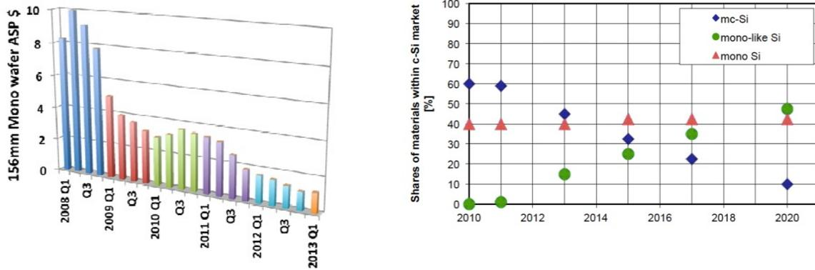
Figure 2. (a) Quarterly ASP of mono 156 nm quasi-square Si wafers 2008-2013 (various sources); (b) International Technology Road Map (ITRPV) market share projections of mono and mono-like wafers (March 2012).
