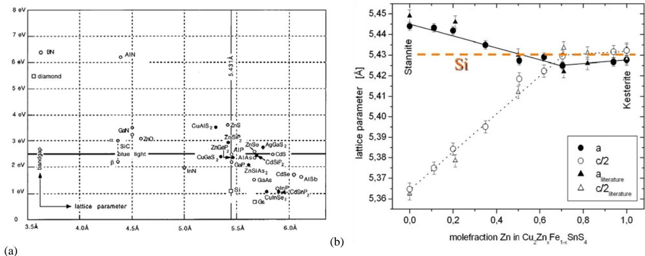
Figure 5. (a) Bandgap versus lattice parameter of a range of semiconductor compounds [6]; (b) Lattice match to kesterite and stannite.
