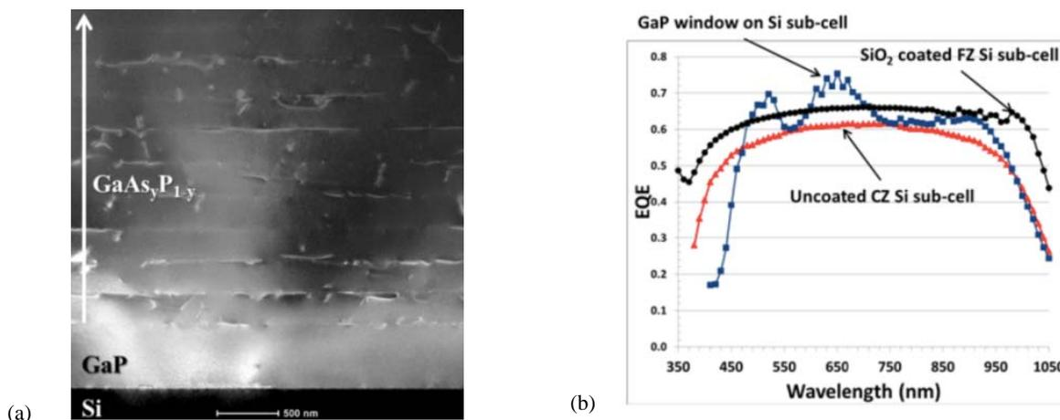
Figure 3. (a) Cross-sectional dark-field STEM image of an MOCVD  $\text{GaAs}_{0.7}\text{P}_{0.3}$ /step graded  $\text{GaAs}_y\text{P}_{1-y}/\text{Si}$  structure [2]; (b) EQE for CZ Si sub-cells with and without a GaP epitaxial front window. Also shown is the improved infrared response of a FZ Si bottom layer cell developed for this work [2].
