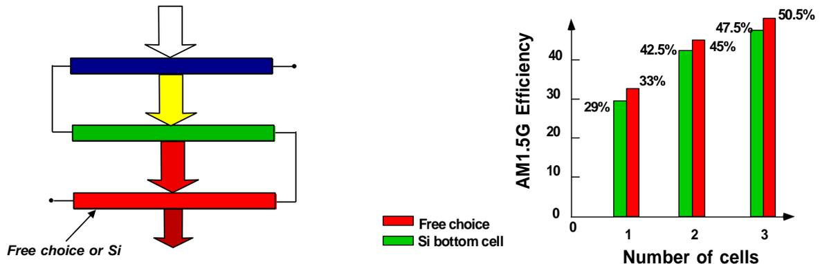
Figure 1. Tandem cell stack and limiting efficiency, with (green) and without (red) the bottom cell constrained to be silicon.
