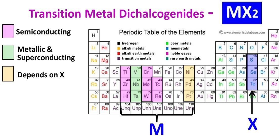
Figure 2. The transition metal di-chalcogenides are an example of 2D layered materials. Depending on the combination of the transition metal M, and the chalcogen atom X (S, Se, Te), a wide range of properties can arise.
