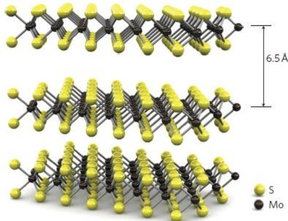
Figure 1. Crystalline structure of layered MoS<sub>2</sub> where the Mo atom is sandwiched between the S atoms. The interlayer bonding occurs via the weak van der Waals interaction. Unlike graphene, monolayers of MoS<sub>2</sub> exhibit a large band-gap ~ 1.8eV and it is also a direct-band gap semiconductor.
