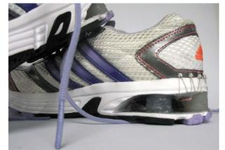
(2) To get the most out of a DEG, its mechanical strain should be sensed. The best way to do this is to monitor the elastomer directly: to self-sense. The DEGs can now self-sense, simultaneously harvesting energy and sensing mechanical state without the need for bulky sensors.
