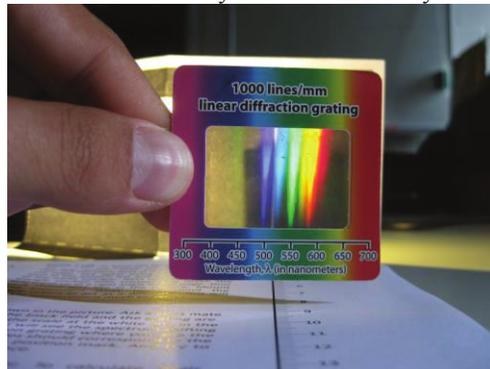
Figure 3 Colours of the spectrum of an energy saving light bulb seen through a diffraction grating provided in the kit
