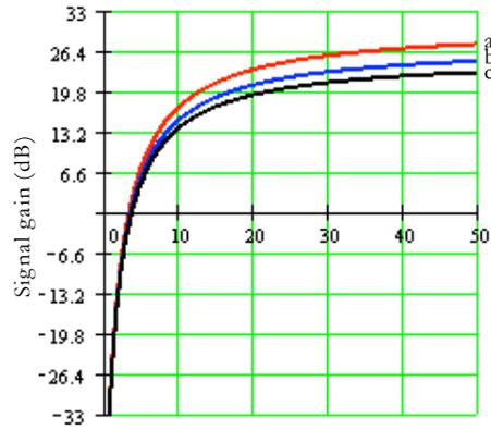
**Fig. 1.** The variation of signal gains versus launched pump powers for the signal power regime  $50 \mu\text{W}$ . (a), (b) and (c) curves correspond to  $-20 \text{ }^\circ\text{C}$ ,  $20 \text{ }^\circ\text{C}$  and  $60 \text{ }^\circ\text{C}$ , respectively.  $\tau$  is taken as  $10 \text{ ms}$  and  $L = 15 \text{ m}$ .
