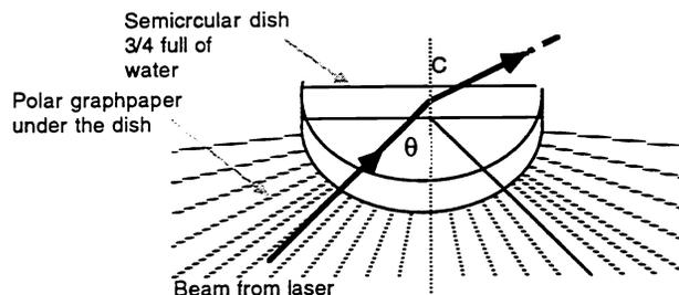
Fig 6. Total internal reflection in a semi-circular dish.
