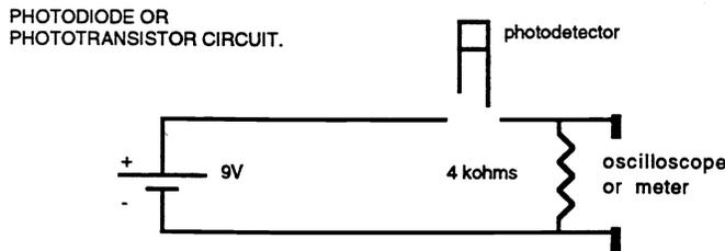
Fig 7. The reverse-biased photo-detector circuit.
