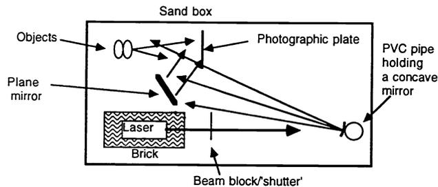
Fig 23. Standard transmission hologram-making system.
