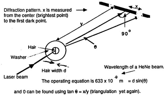
Fig 20. Measuring the diameter of a human hair by studying diffraction patterns.
