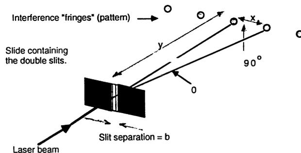
Fig 19. A double slit interference experiment.
