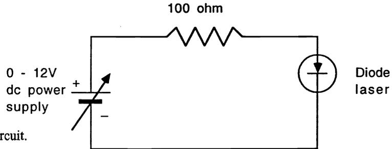
Fig 24. A visible laser diode circuit.
