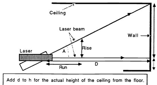
Fig 1. Measuring the height of a room.
