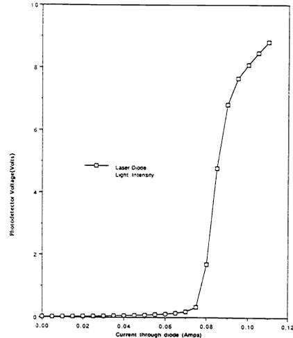
Fig 25. The light emitted by a visible diode laser v current.
