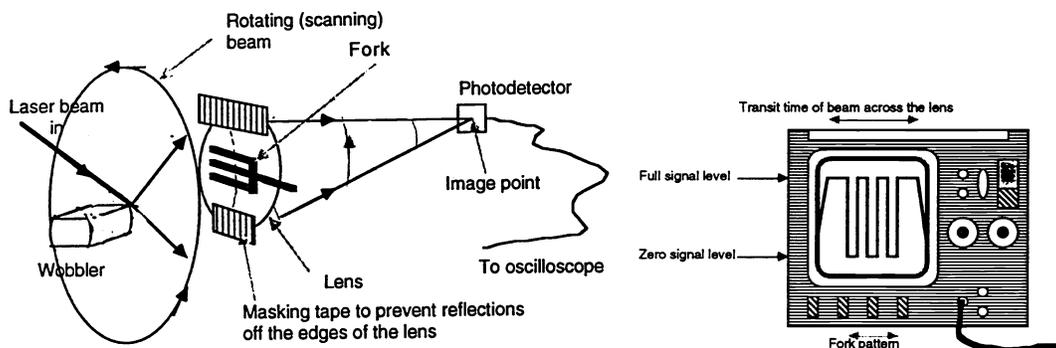
Fig 13. "Reading" a simple pattern with a scanning system. Fig 14. The oscilloscope pattern.
