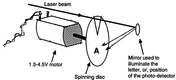
Fig 15. The laser beam "chopper".
