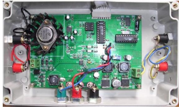
Figure 4. Photovoltaic charging controller.
