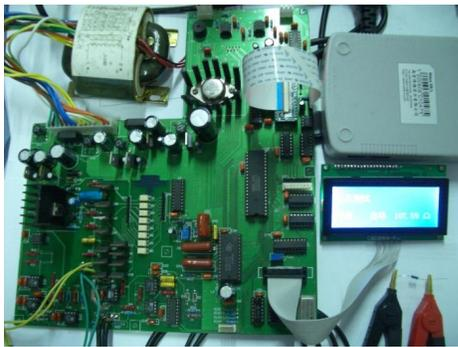
Figure 1. Intelligent DC micro-ohmmeter.
