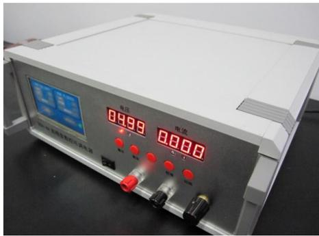
Figure 3. Digitally-controlled high-precision DC power supply.
