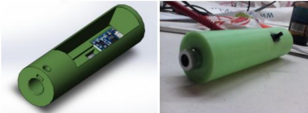
Figure 7. The source's shell, made by 3D-printing
