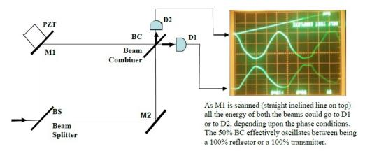
Figure 2.1.2. **Left diagram:** the same scanning MZI as in Fig.2.1. **Right diagram:** An oscilloscope snap shot of the scanned intensity variation in the two output ports of the interferometer. It is clear that one the intensity registered by D2 is minimum, that due to D1 is maximum.
