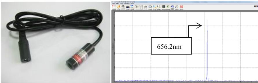
Figure 6 Light source and spectrum of red semiconductor laser
