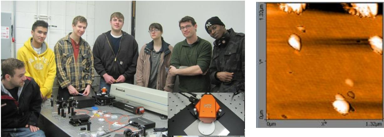
Figure 6. LEFT: Monroe Community College students during an AFM lab. (A small orange-color AFM and its controller (black) are located at the left side of the picture). INSERT: A magnified picture of an AFM. RIGHT: Typical unprocessed AFM micrograph of nanodiamonds.
