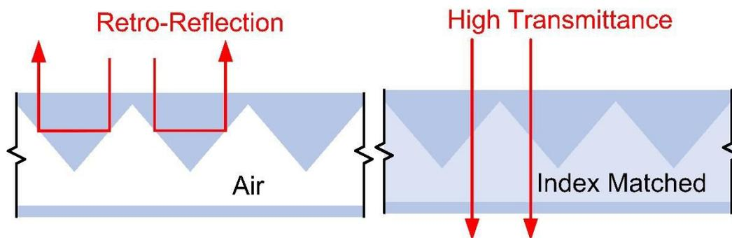
Figure 1: Drawing of our published Smart Glass panel, consisting of cavity behind solid corner-cube retroreflector array. When cavity is filled with index-matching fluid, structure switches from reflective to transparent.
