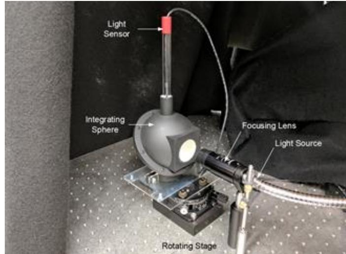
Figure 5: Experimental setup for measuring transmission of TIR smart glass designs vs. angle of incidence.
