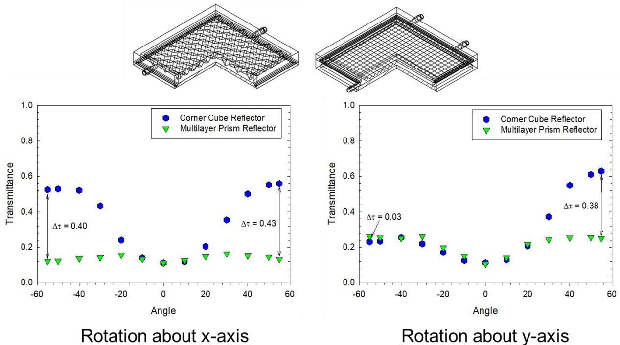
Figure 6: Measurements of the transmission vs. angle of incidence (with air in the cavities) of the published corner-cube design (blue) and crossed-prism design (blue), with angle of incidence along x and y axes.
