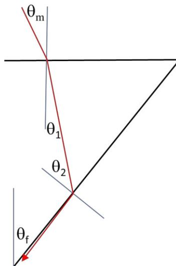
Figure 3: Ray incident on solid corner-cube retroreflector at TIR condition for first facet.
