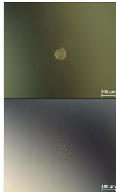
**Fig. 2: Typical damage morphologies on E-BEX coating samples: Image (a) correspond to defects appeared after 2 shots at 26.3J/cm<sup>2</sup> on sample 1C28 and Image (b) correspond to defects appeared after 2 shots at 26.3J/cm<sup>2</sup> at 14.3J/cm<sup>2</sup> on sample 1C30.**
