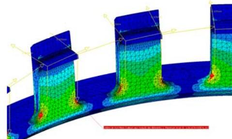
**Fig. 4: FEM analysis - Thermo-elastic case**
