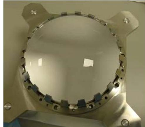
**Fig. 3: L3 Lens assembly**
