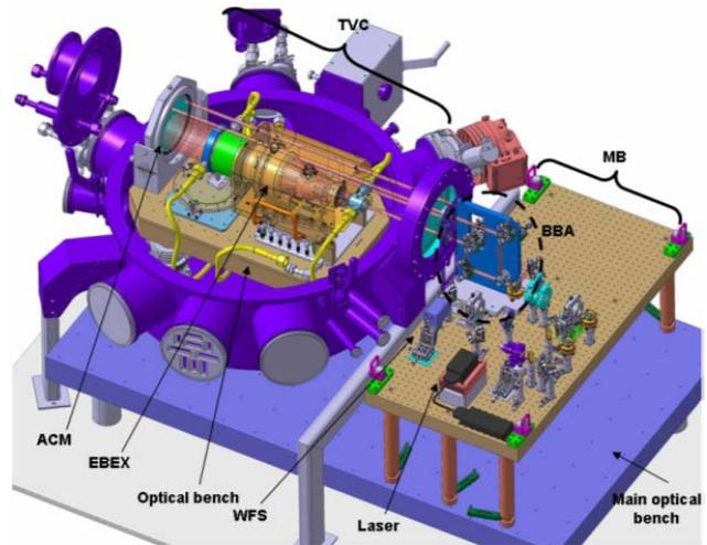
**Fig. 10: E-BEX in its testing environment**
