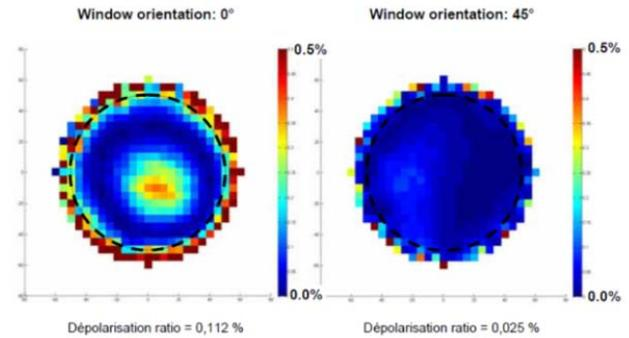
**Fig. 8: Window depolarization mapping**
