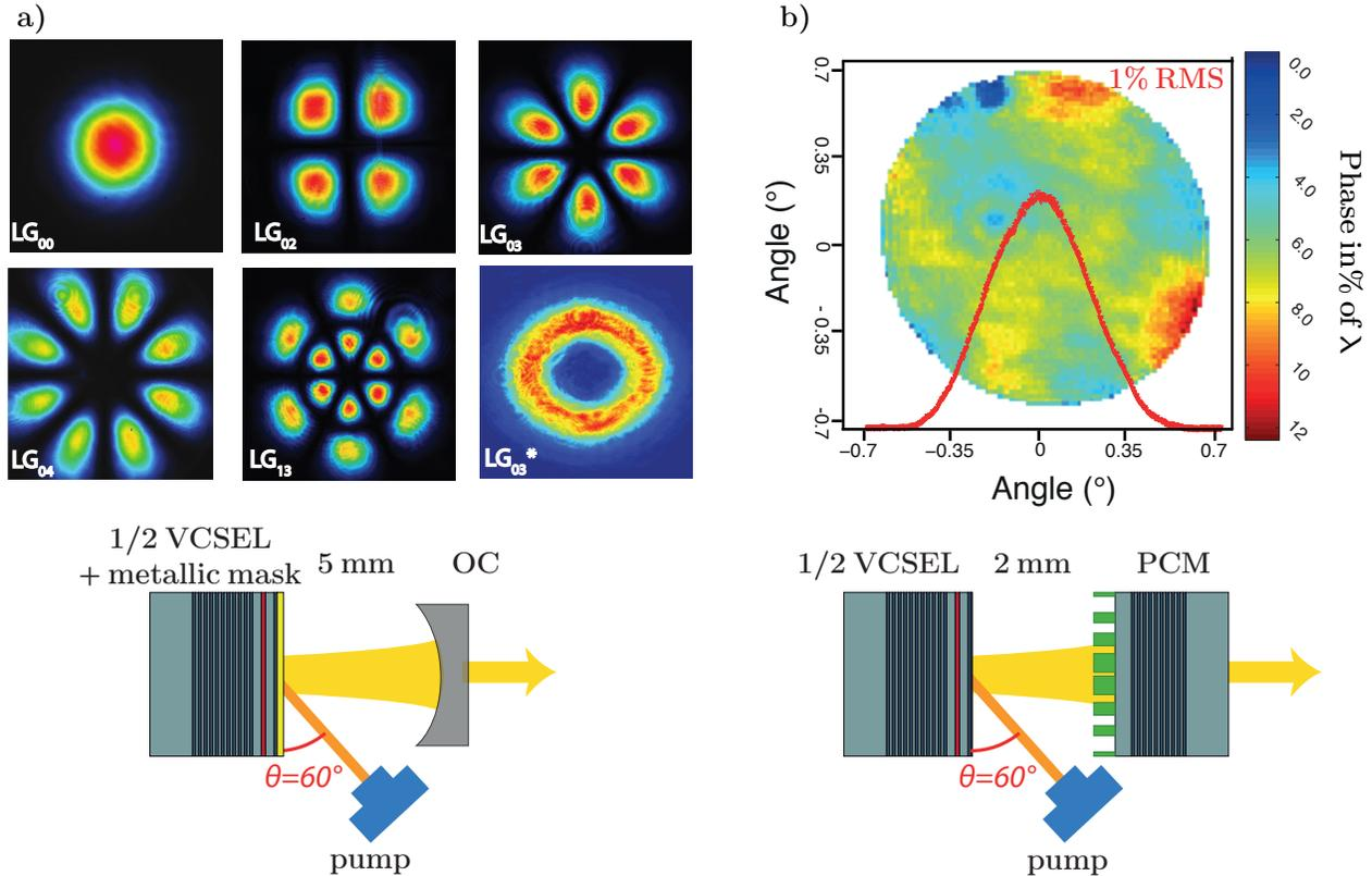
Figure 3. a) High order degenerated and non-degenerated Laguerre-Gauss modes obtained experimentally with metallic masks and a 5mm VCSEL cavity. b) Optically stable aberration-free VCSEL cavity based on planar technology thanks to the transverse control of the phase inside the laser cavity thanks to the photonic-crystal mirror technology.
