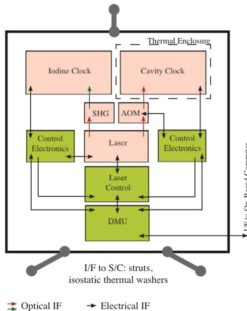
**Fig. 5.** Functional diagram of the mSTAR scientific payload.
