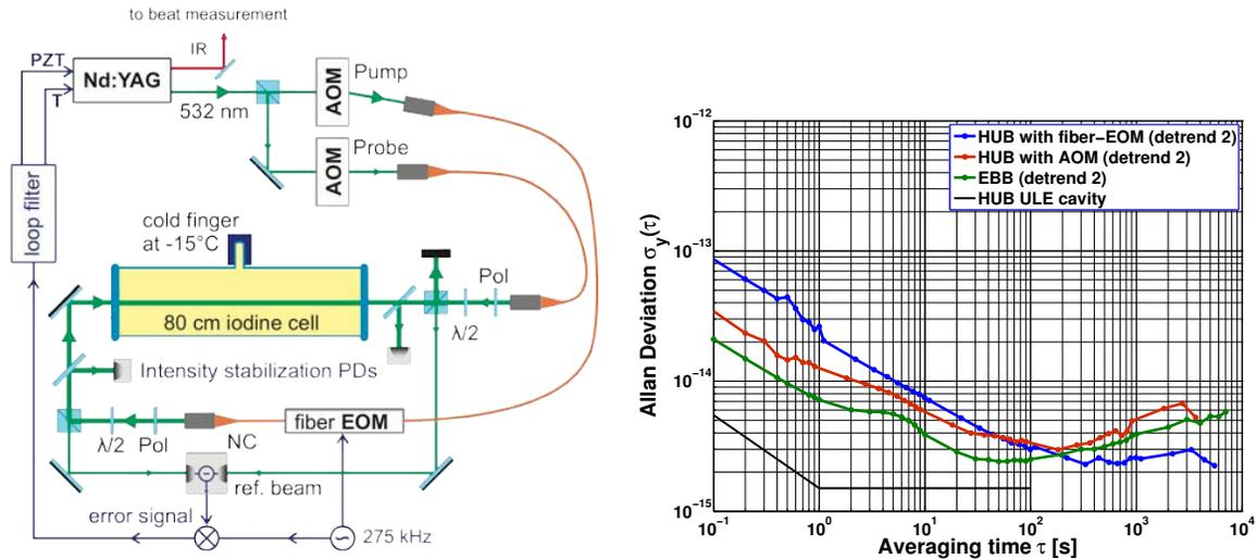
**Fig. 1.** Left: Schematic of the laboratory setup of the iodine frequency reference at the Humboldt-University Berlin [6]. Right: Frequency stability of iodine-based frequency references [6]. The blue curve corresponds to the HUB laboratory setup as presented in section I using a fiber EOM for phase modulation. The red curve corresponds to a similar setup using an AOM for phase modulation. The green curve shows the frequency stability of the EBB setup as detailed in section II.
