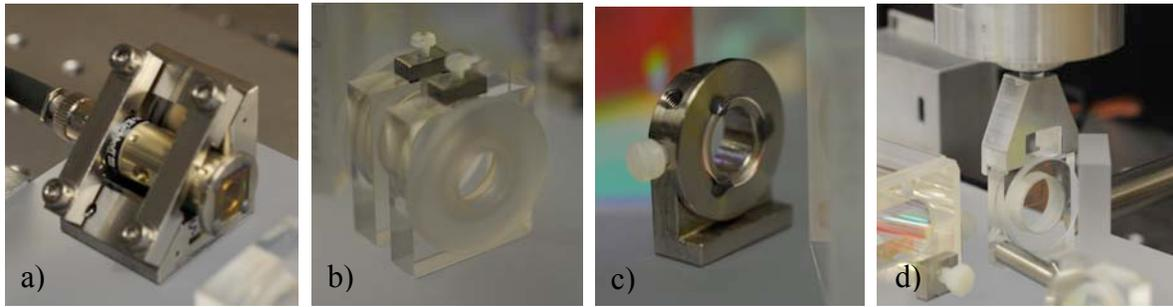
**Fig. 4.** Detail photographs of the fiber collimator with Invar mount and polarizer (a), the pair of wedged glass plates (Risley prism pair) with all-glass mounts (b), the waveplate with titanium mount (c), and a lens mounting during integration process (d).
