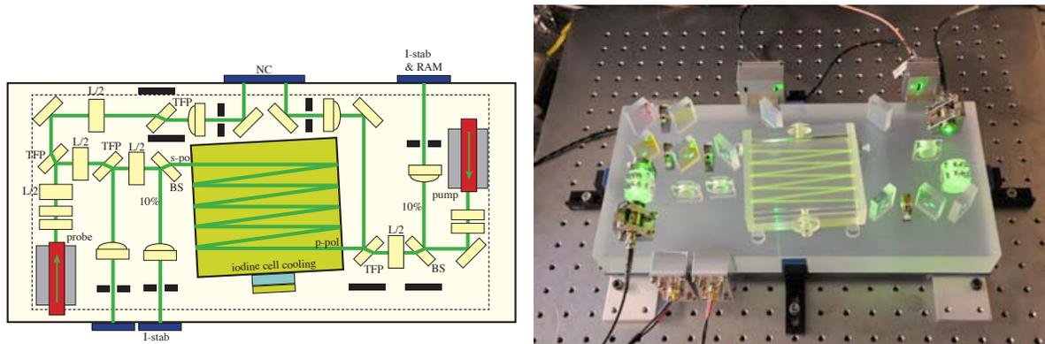
**Fig. 3.** Schematic and photograph of the spectroscopy setup developed on engineering model level using an 18 cm x 38 cm baseplate made of fused silica.
