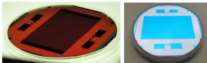
Fig. 6. VNIR filter wafers with 110 mm diameter. The filter stripes are the long rectangular stripes on the wafer. The surrounding larger filter zones are coupon regions used for testing
