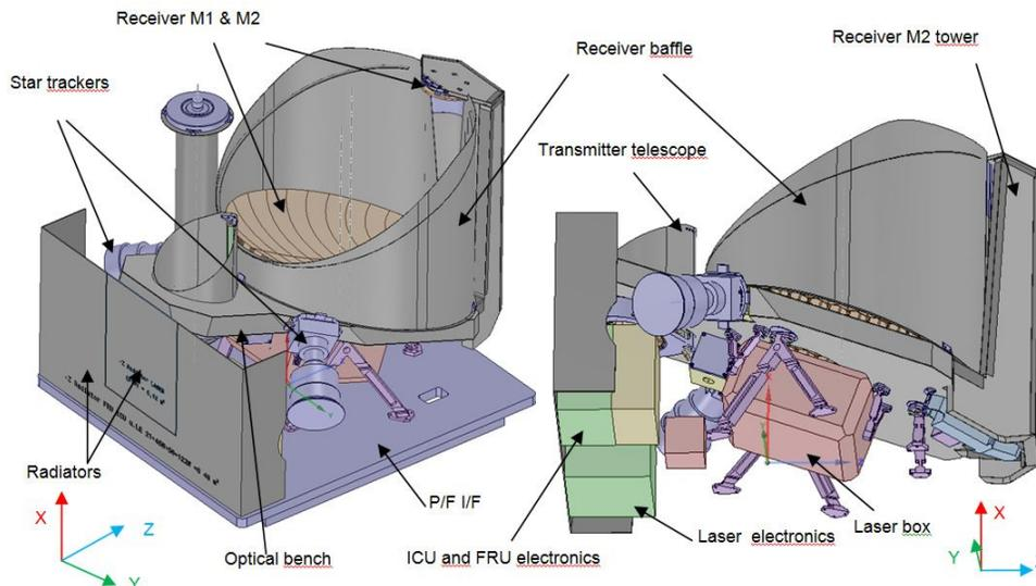
**Fig.1:** MERLIN payload accommodation
