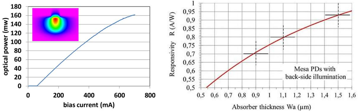
Fig. 2. (left) DFB experimental results from various devices within the 1<sup>st</sup> fabrication run and (right) simulation of the back-side illuminated UTC photodiode versus absorber thickness ( $W_a$ )
