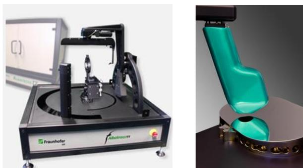
Fig. 2. Left: Table Top System *AlbatrossTT*, Right: Light Scattering Sensor *horos*
