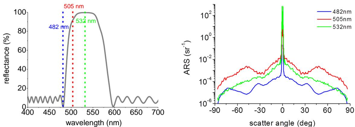
Fig. 9. Rugate filter. Left: Spectral properties. Right: Angle Resolved Scattering at different wavelengths.
