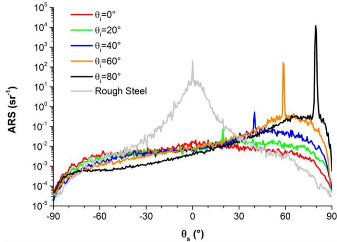
Fig. 4. Scattering of Acktar black coating for different angles of incidence at 4.6  $\mu\text{m}$
