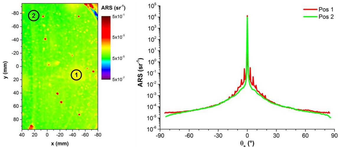
**Fig. 3.** Surface inspection of aluminum mirror using light scattering at 532 nm.
