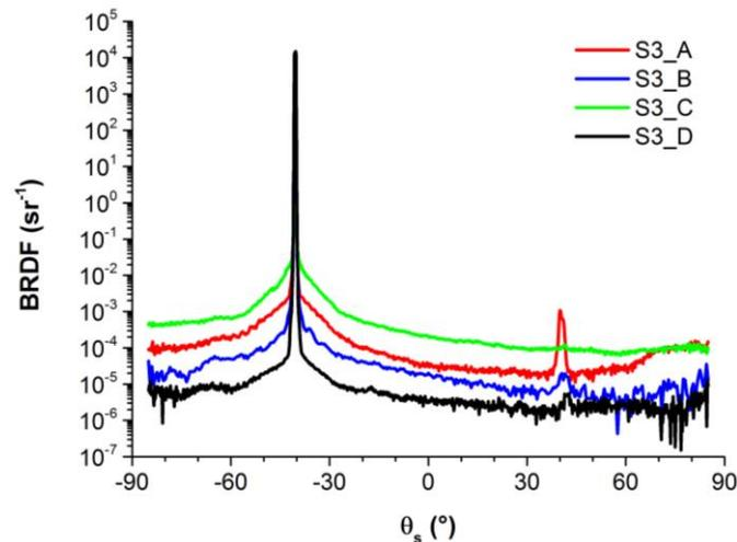
Fig. 8. Scattering of different samples of mirror S3
