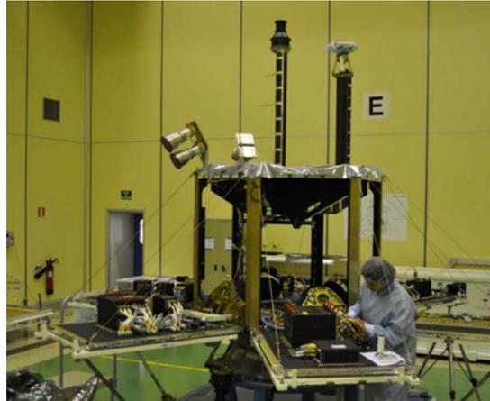
**Fig. 2.** SEOSAT/Ingenio Flight Platform under integration (Courtesy of Airbus Space & Defence)
