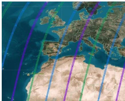
**Fig. 1.** SEOSAT/Ingenio orbit repeat cycle (ground-tracks for three-days coverage )
