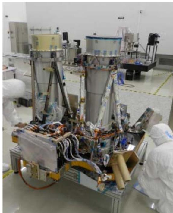
**Fig. 7:** The SEOSAT/Ingenio Primary payload EQM under integration in ISO-6 (courtesy of INTA)
