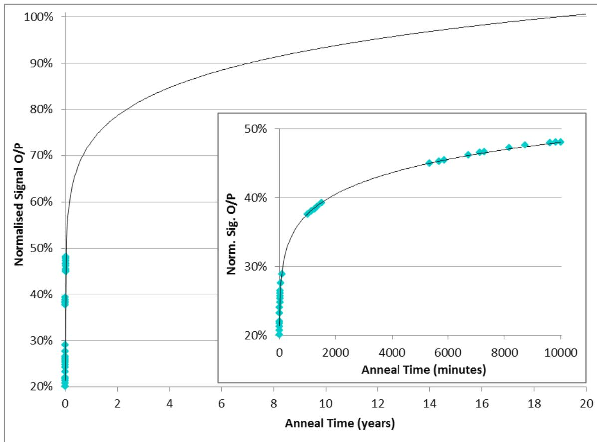
**Fig 3.** Recovering output over 20 years of annealing for A-3. Inset: close up of output vs. anneal time.
