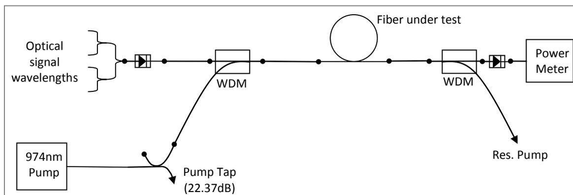
Fig. 1. Single pump EDFA photo-anneal set up
