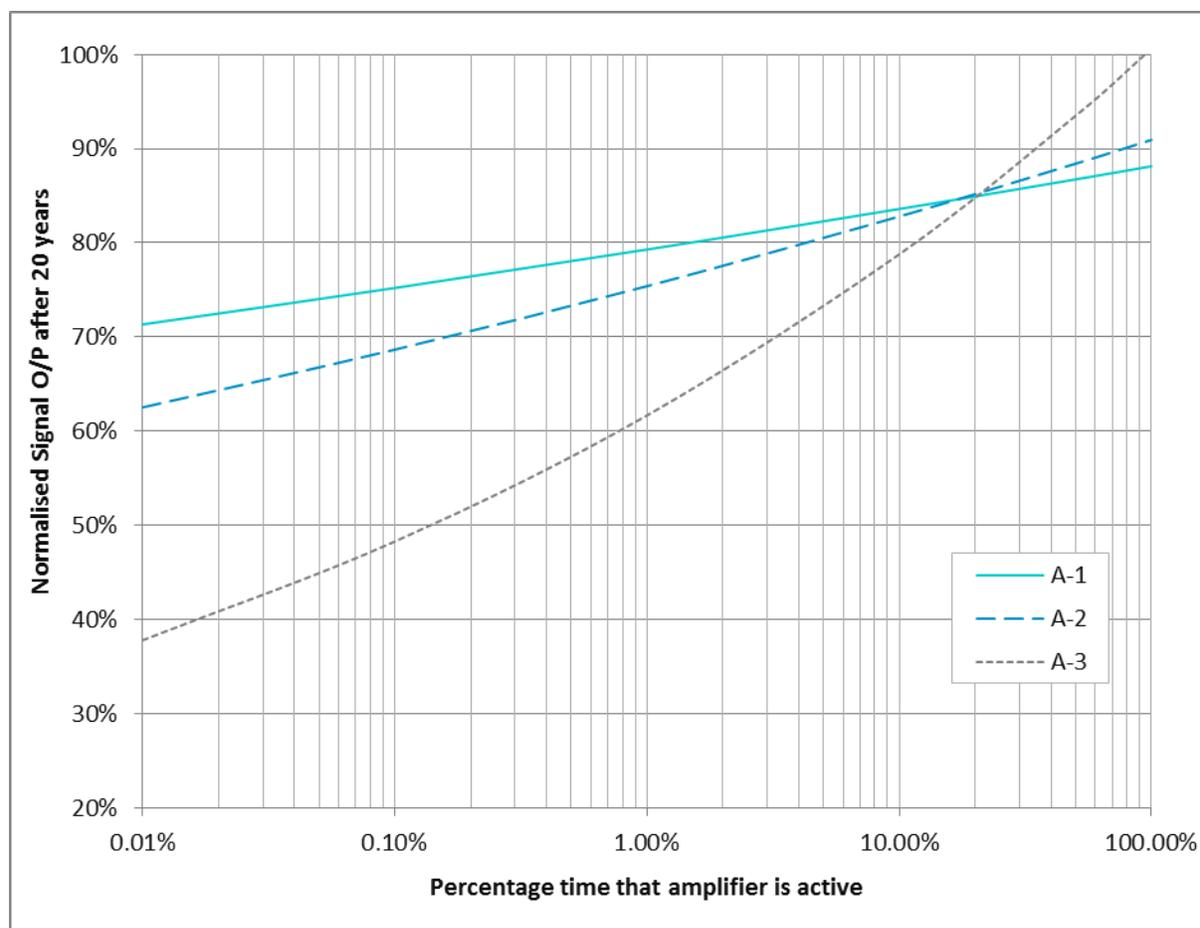
**Fig. 4.** Amplifier output recovery under discontinuous use
