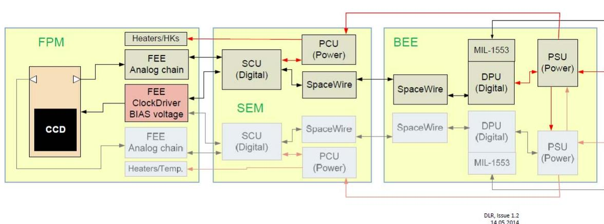
Fig. 4. CHEOPS Electrical sub-system fault tolerance architecture (DLR)
