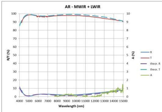
On this measured curve, we have superimposed the theoretical expected curves (dashed lines) and the measured one (solid lines, red for transmittance and blue for reflectance).
