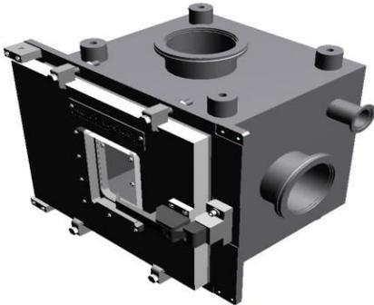
The deformation is measured in ambient conditions, but a dedicated chamber is being prepared to allow a measurement under vacuum to assess the effect of environment.
