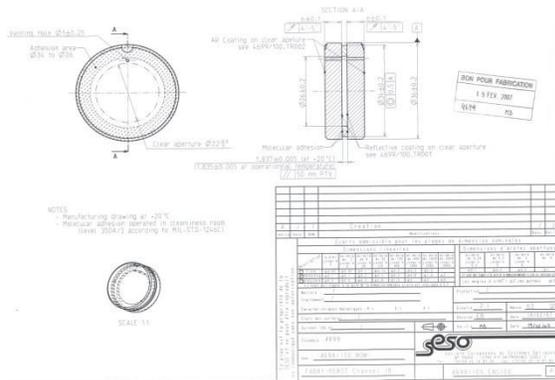
Thales SESO has produced a ZnSe Fabry-Perot unit with specific Rmax and AR Coatings to filter the infrared band  $5\mu-7,7\mu$  (= Channel 1A of MIRI, an experiment for the James Web Space Telescope). Mounting by molecular adherence (= optical Contacting) as well as optical coatings, have been tested successfully down to 20°K (= -250°C)
