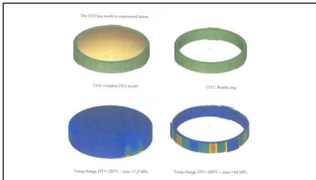
**Fig. 4:** FEM analysis of worst case # 1 = CO2, because lens made out Silica which is a « strong » material with a CTE very far from the one of aluminium )
