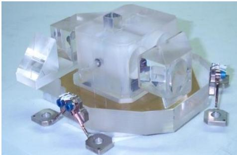
SESO has produced in 2003 a Silica “Double Channel” Fabry-Perot assembly qualified for Space Application. Operating temperature is +20°C stabilised but qualification has been achieved from +60°C down to -40°C. Attachment of the 3 accurate FP plates and spacer (accuracy in the range of  $\lambda/100$ PTV) was using optical contacting process (or molecular adherence)
