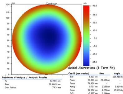
The deformation induced by the coating is identified to be about 70 nm concave (on a clear aperture of 124 mm). The AR coating induces tensile stress in the layers. The plate was wedged to minimize the ghost images in the optical layout. The effect of the wedge on the measured deformation is limited, but not null: this is the reason why we observed a 9 nm astigmatism value oriented along the wedge direction
