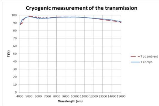
The same previous samples (figure 11) were measured also at liquid nitrogen temperature (inside Dewar at  $-196\text{ }^{\circ}\text{C}$ ).
