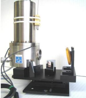
The Dewar can be adapted onto our 12° absolute reflectance accessory. Connected to a controller, it can also allow heating the sample in high temperature conditions (up 350°C) to allow measurements in good conditions. The Dewar is equipped with ZnSe windows which are heated to avoid condensation. The cell can be brought to vacuum using a convenient connection to a pumping system. It can also be used under dry nitrogen for simpler configuration.
