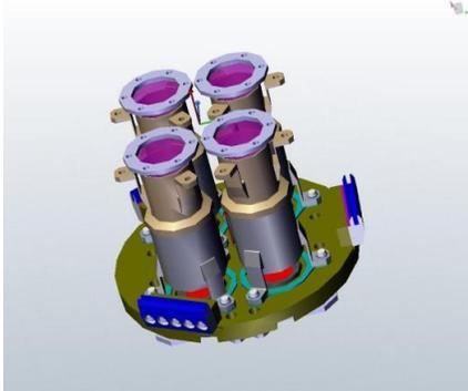
After being spectrally separated and collimated, the NIR/IR optical beams reach the cold optics, which are located inside a common cryostat.
