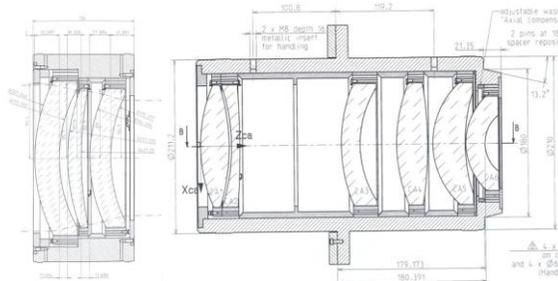
**Fig. 3:** EMIR collimator (on left) and camera (on right)
