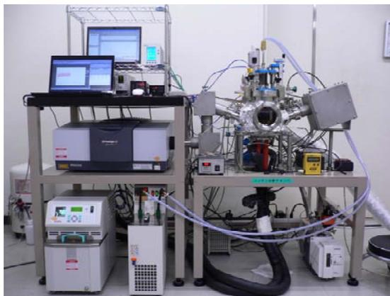
Fig. 3. In-situ Contamination Spectroscopic Analysis Chamber.
