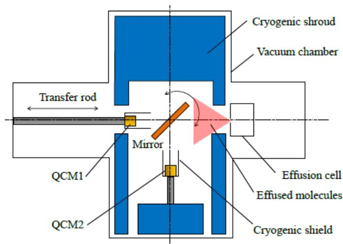
Fig. 1. Diagram of the facility.
