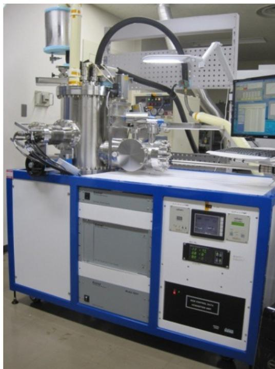
Fig. 2. Outgassing rate measurement equipment in JAXA.
