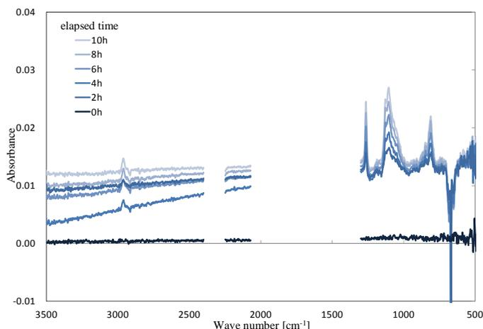
**Fig. 4.** FT-IR spectral absorbance overlaid with the spectrum of each time elapsed (Bakeout at 125°C)
