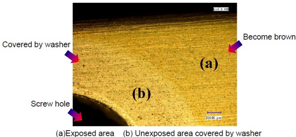
**Fig. 5.** Picture of the aluminum alloy frame surface becoming brown except for the unexposed area covered by washers.
