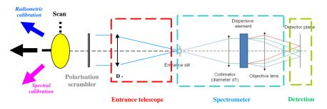
Figure 2. Components of the instrument's functional system
