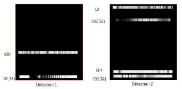
Figure 7. Example of the echelle spectrometer with double mutiplexing that allows the observation of 6 bands with only two detectors. The black areas are the sensitive areas of the detectors. The strips are the spectrum associated to each spectral band.
