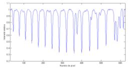
Figure 5. Example of an experiment profile for the CO<sub>2</sub> spectrum in band B2 (uncalibrated)
