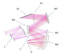
Figure 10. Optical diagram of the spectrometer with cross-
