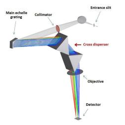
Figure 8. Principal scheme of cross-disperser grating.
