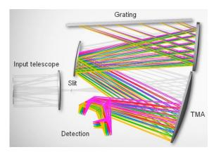
Figure 3. Illustration of spectral axis versus spatial axis
