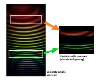
Figure 9. On the left, classical image of echelle spectrum complete. On the right, possibility to group together several narrow spectral band on one detector thanks to the double multiplexing.
