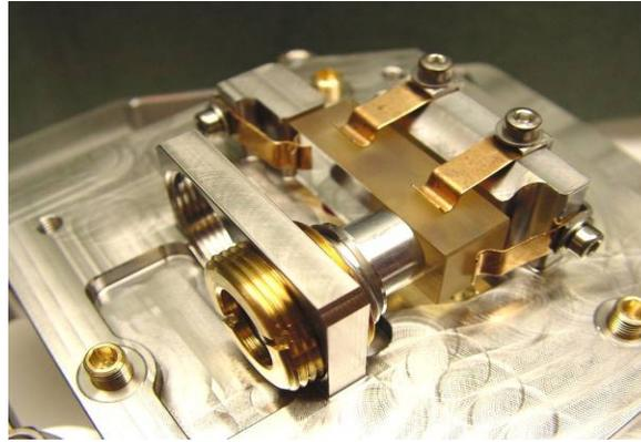
**Fig. 8.** Cryogenic vacuum CTE measurement setup
