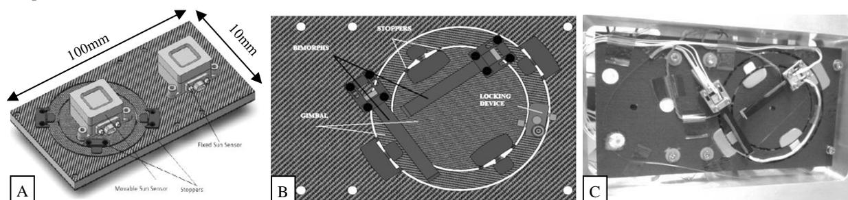
**Fig. 2.** A) concept design of Optical Bench, frontside, B) concept design of Optical Bench, backside, C) Assembled Optical Bench
