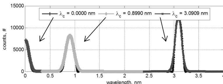
Fig. 6. FBG peak measurements
