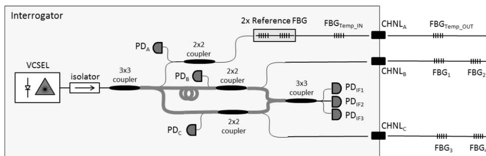
Fig. 4. Schematic drawing of interrogator
