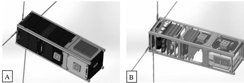
**Fig. 1.** Nano-Satellite model, A) outside (dimension 30x10x10cm), B) inside
