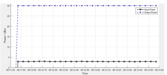
Figure 10: EDFA operation onboard BIROS (Input & output power)
