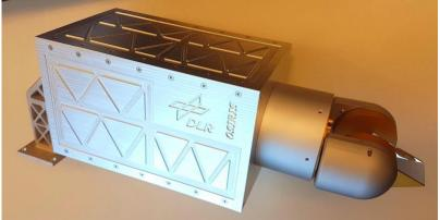
Figure 8: Mock Up of third generation OSIRIS terminal
