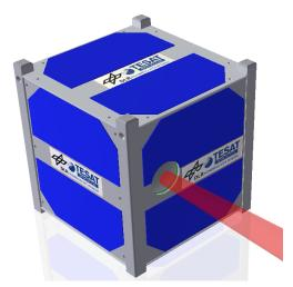
Figure 6: Illustration of CubeSat with OSIRIS terminal installed
