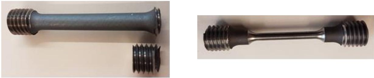
**Figure 3** Change of sample design required due to notch effect (left: old design, right: modified shape Type B), built process 1 and 2
