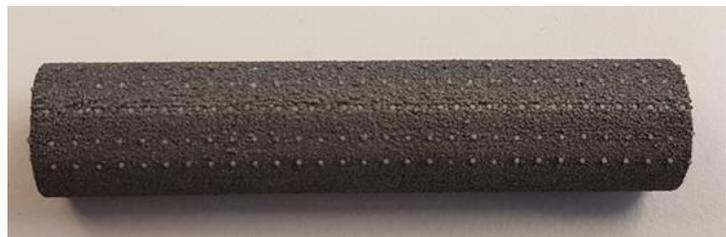
**Figure 4** Change of support structure design for built process 3 due to failure of horizontally built tensile test samples (built process 3)
