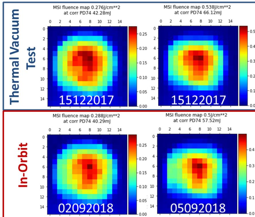
Figure 1: Laser beam profile estimate from on ground tests (blue frame, top panel) and in flight (red frame, bottom panel). Predicted peak fluence and emit energy are provided at the top of each image. Left column shows 40mJ, right column around 60mJ emit energy.
