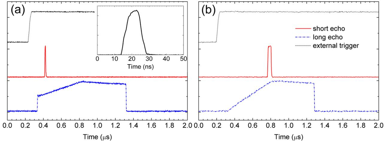
Figure 5. (a) Short pulse: 10 ns, shift 80 ns, long pulse: 1000 ns, initial amplitude  $p_1 = 50\%$ , flat part  $p_2 = 50\%$  of the pulse width, external trigger with 10 kHz repetition rate. Inset shows the short pulse. (b) Short pulse: 40 ns, shift 500 ns, long pulse: 1000 ns, initial amplitude  $p_1 = 1\%$ , flat part  $p_2 = 50\%$  of the pulse width, external trigger with 10 kHz repetition rate.
