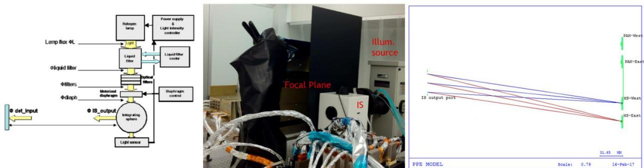
Figure 4. Diagram (left) and image (center) of the used FP radiometric set-up; right: optical FP model corresponding to this test configuration.
