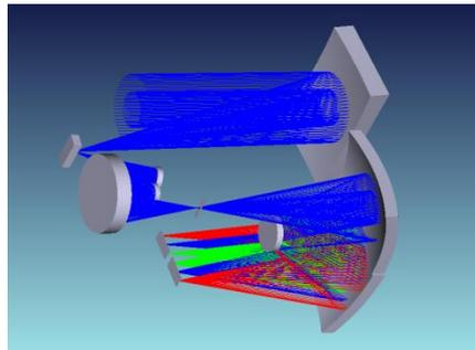
Fig.2. Optical system layout of visible and infrared imaging spectrometer
