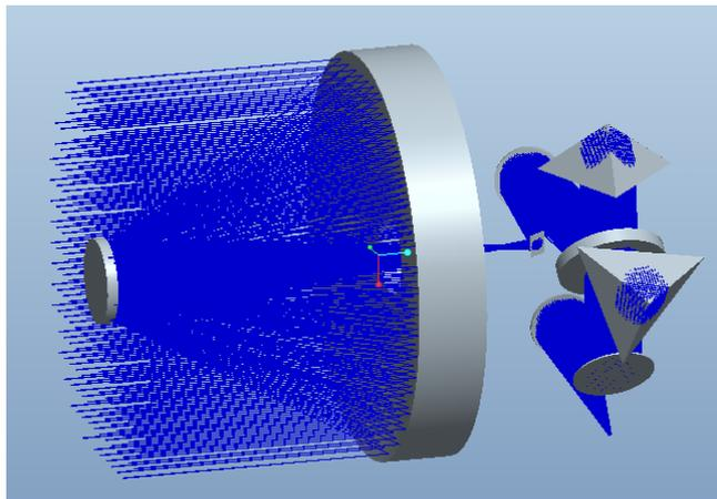
Fig.3 Optical system of thermal emission spectrometer
