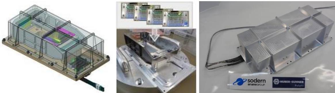
Figure 8. OPTIMA Optical Switch Breadboard: design integration and full integrated Elegant Breadboard.
