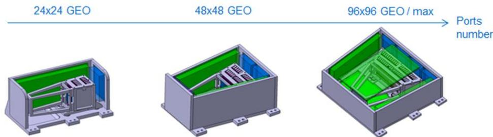
Figure 12. Optical Switch future concepts of mono-bloc implementation from 24x24 ports to 96x96 ports.
