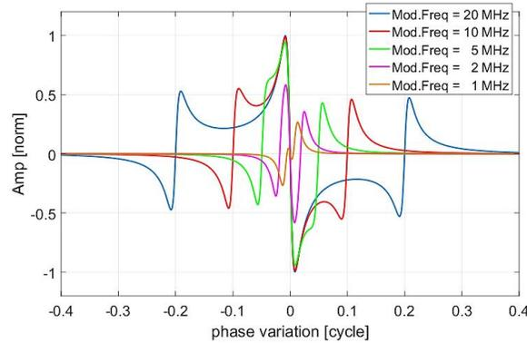
Figure 3. Error signal shape for the ideal case,  $FSR = 100$  MHz,  $R = 0.1$
