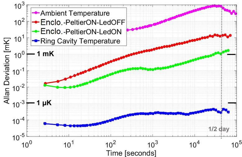
Figure 17. Allan deviation of ambient temperature, enclosure temperature and ring cavity temperature. Magenta curve: deviation of ambient temperature; red curve: deviation of enclosure temperature when LED current controller was off; green curve: deviation of enclosure temperature when LED current controller was active; blue curve: deviation of ring cavity temperature, obtained from beatnote frequency measurement. Enclo: aluminum enclosure.
