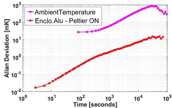
Figure 11. Allan deviation of ambient temperature and enclosure temperature when Peltier locking is activated
