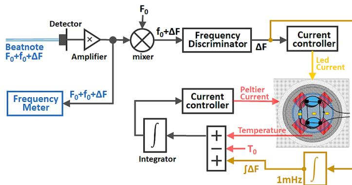
Figure 12. Block drawing of ring cavity temperature control system with 3 channels
