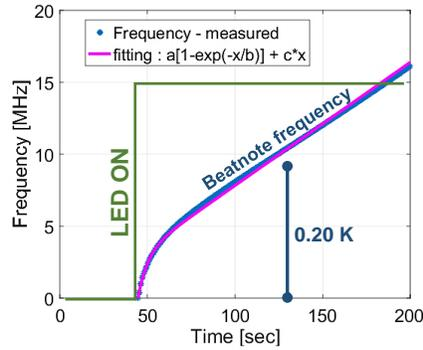
Figure 15. Temporal response at long time range of ring cavity temperature
