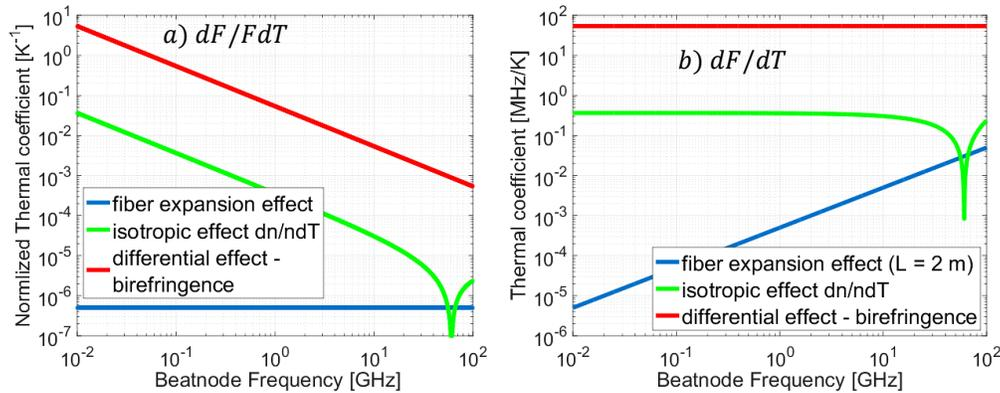
Figure 5. a) Fractional thermal deviation of beatnote frequency ( $dF/FdT$ ) following beatnote frequency  $F$
