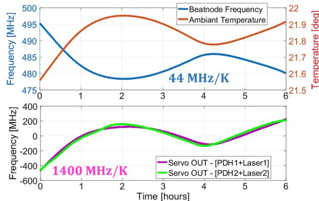
Figure 7. Experiment: simultaneous recording of the ambient temperature and beatnote frequency (upper graph), and of the correction signals of the two lasers, converted into optical frequency (lower graph).
