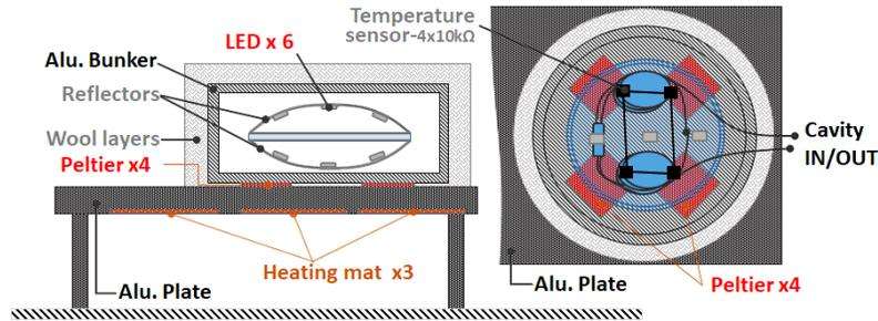
Figure 8. Fiber ring cavity mounted in the  $\varnothing=200$  mm thermal enclosure
