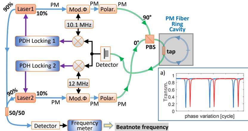
Figure 6. Double laser lock (Pound Drever Hall scheme) on a fiber ring cavity.
