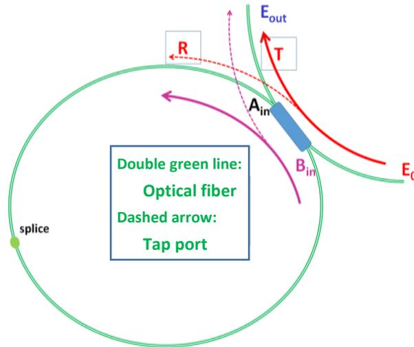
Figure 1. The fiber ring cavity - obtained by fusion splicing the two tap ports of a low-ratio PM coupler
