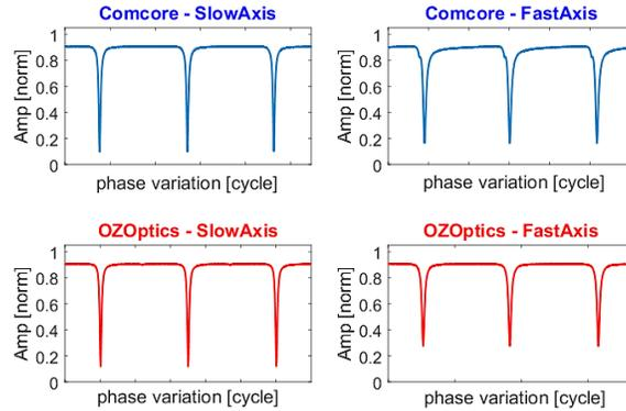
Figure 2. Measured transmission through the resonators obtained from ComCore and OzOptics couplers.
