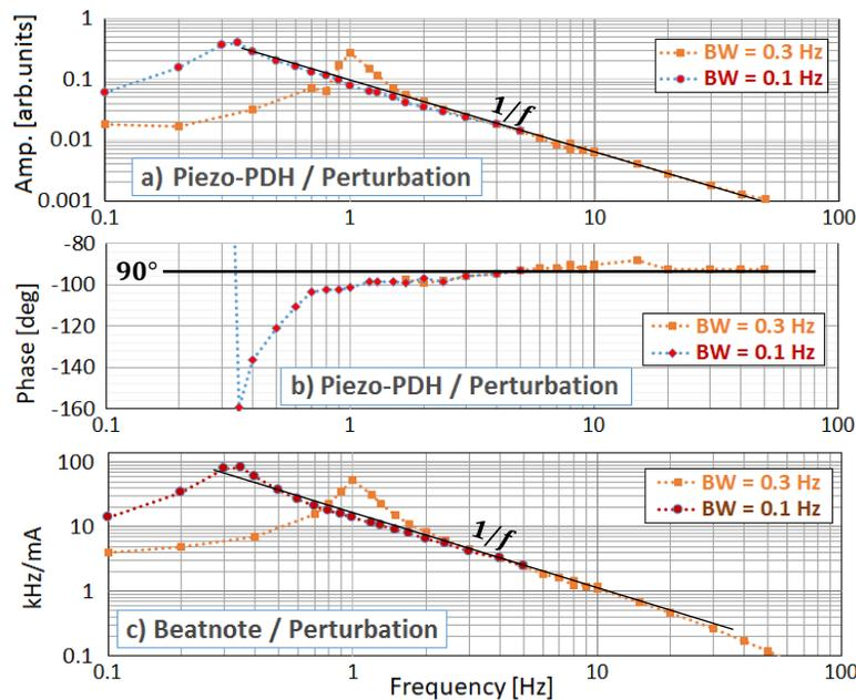
Figure 16. Transfer function shapes of PDH piezo correction & beatnote frequency versus LED current
