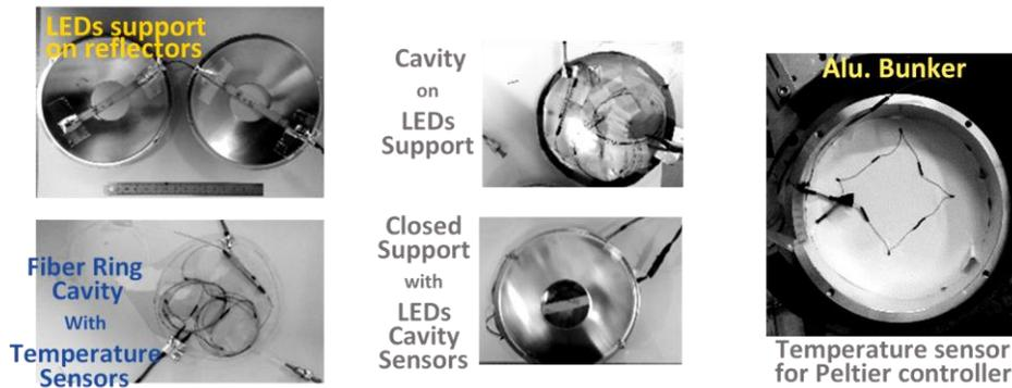
Figure 9. Mounting fiber ring cavity and six LEDs between two reflectors
