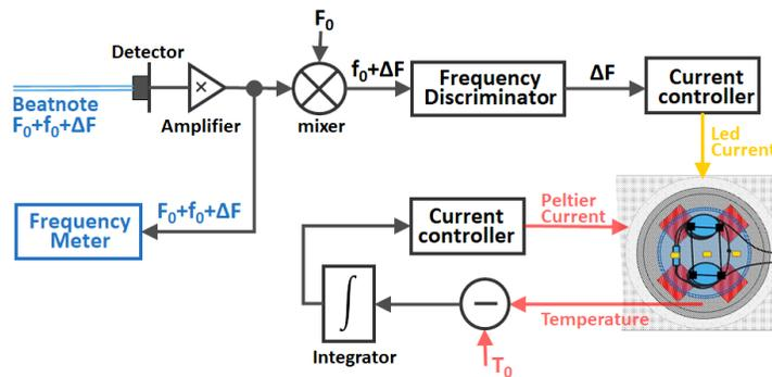
Figure 10. Block drawing of the ring cavity temperature control system with two channels for beatnote frequency measurement
