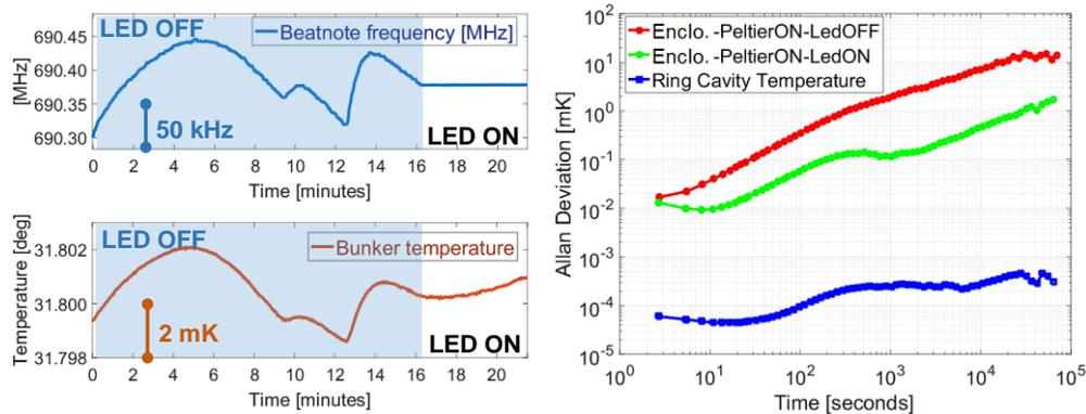
Figure 13. Beatnote frequency raw data and Allan deviation (converted to temperature) before and after activation of LED locking system
