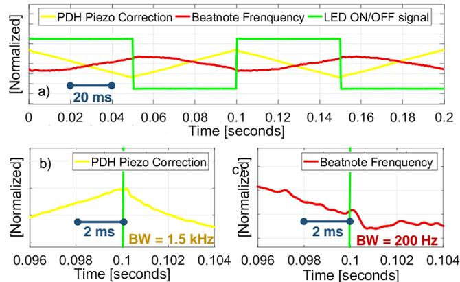
Figure 14. Beatnote and optical laser frequency variation when turning LEDs on/off at 10 Hz
