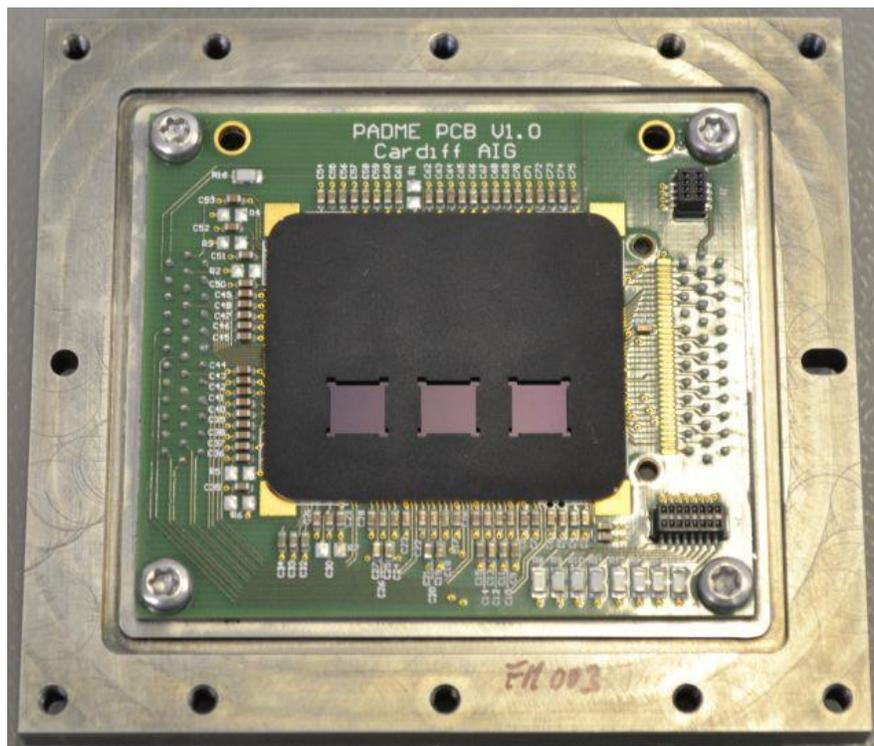
Figure 9: Test detector for initial performance test.
