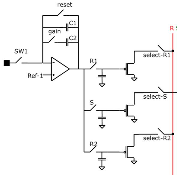
Figure 2: basic topology of a CTIA pixel cell.
