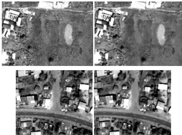
Figure 5 - Restoration results on two extracts of a PAN PHR image: restored images with the current ground segment (left), and with the new restoration pipeline (right). One can see on uniform areas that noise has been well removed, compression artefacts have disappeared and edges are better preserved on the right.
