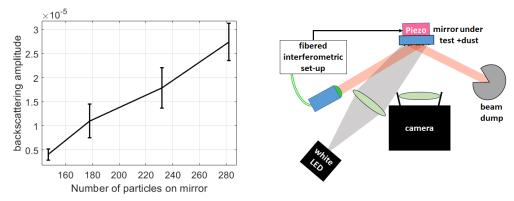
Figure 9. Left: the dependence of the fractional backscattering  $\sqrt{b_s}$  on the number of particles at the surface (preliminary results). Gaussian size of the laser beam: 1.71 mm. Backscattering is measured in parallel polarization. Right: coherent backscattering measurement set-up for the dust-contaminated mirror.
