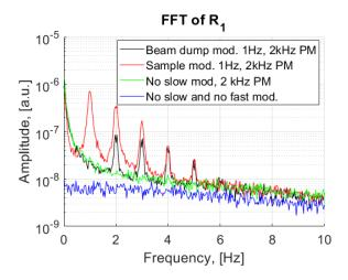
Figure 3. FFT of  $R_1$  when slow (1 Hz) modulation is applied to the beam dump (black), and the case without slow modulation (green). For the sample modulation (red) we had adjusted the voltage to reach the condition  $J_0(\delta) = 0$ . The case when neither the fast, nor the slow is applied gives electronics plus laser noise level (blue).
