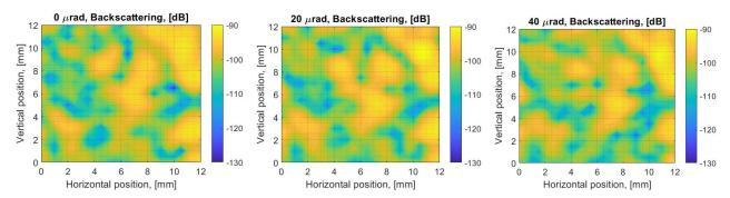
Figure 5. 2D maps of the backscattered power (in dB) of the same scanning area with slightly different incidence angle (20 µrad steps). Incidence angle is approximately 14°. Horizontal and vertical scan step is 0.5 mm. dB is for the fraction of optical power of the backscattered light recoupled into the fiber.
