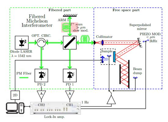
Figure 2. Coherent backscattering measurement setup. Green: optical fibers. Red: free space beams. Dashed red: backscattered light from the sample.
