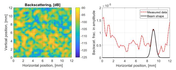
Figure 6. Map of backscattered light with a collimator of 8mm focal length. Size of scattering peak is same as Gaussian beam size ( $\omega_0$ =0.65 mm), in black.
