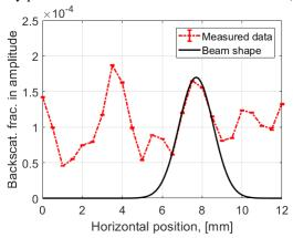
Figure 4. Profile of backscattered light from a moderately scattering target. Black curve (arbitrary units): plotted for comparison, a gaussian beam profile of the same gaussian beam size ( $\omega_0$ =1.71 mm) as the incident beam.
