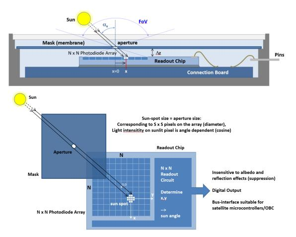
Figure 7: Illustration of the digital sunsensor chip applied in the IBIS sunsensor.
