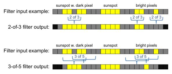
Figure 8: pixel majority voting principle, 2 out of 3 and 3 out of 5
