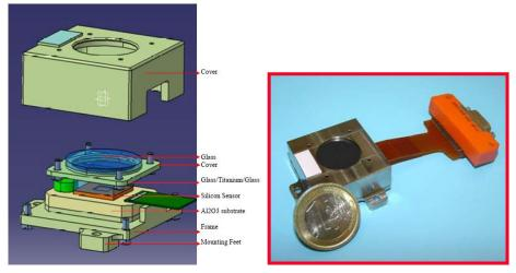
Figure 5: Galileo mini-DSS [3]
