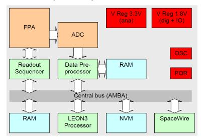
Figure 4: Intended functionality of the LCMS chip [3]
