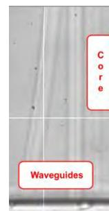
Fig. 1c. Bridging waveguides in single-core fibre cladding
