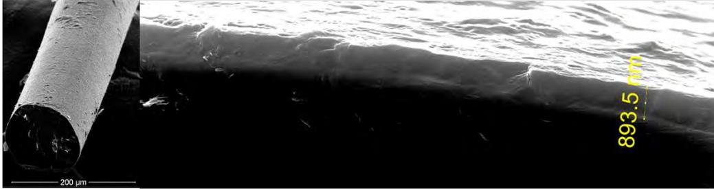
Figure 6: Spinel coated sapphire fiber. Magnified image showing the spinel film on fiber.
