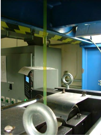
*Figure 3; a glass redraw apparatus*
