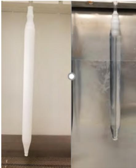
Figure 2b; a CVD-produced soot blank before (left) and after its consolidation into a preform (right)
