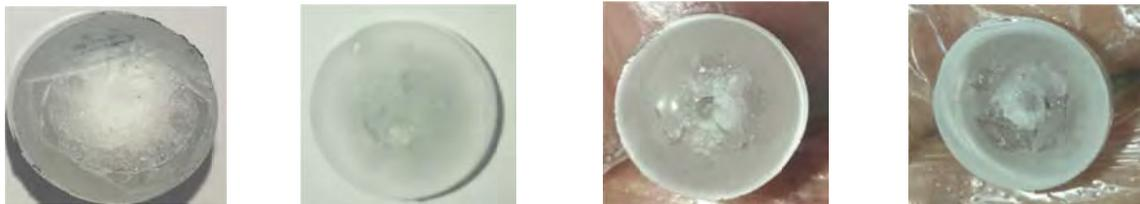
Figure 5. Sliced 3D printed silica fiber preforms showing non-ideal and incomplete cases of silica vitrification. The preforms are sintered at 1600°C for 20 ~ 30 mins.
