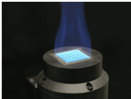
Figure 6: Standard flame burner.
