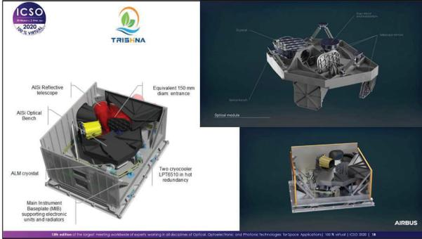
The payload is composed of a VIS/SWIR instrument (ISRO) and a TIR instrument (CNES) shown on the slide with 4 TIR bands from 8,6 to 11.6 microns. Development status of Trishna instrumentation will be presented by CNES/ADS this afternoon in session 6 (paper 267)
